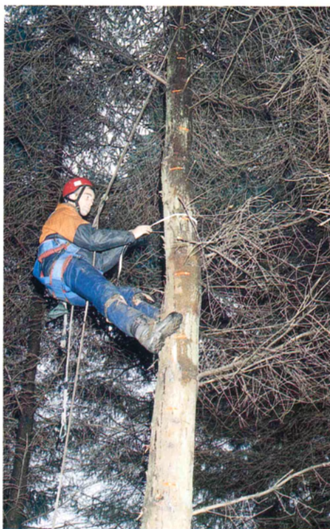
Measuring stem straightness in Sitka spruce in a study to assess log quality (Photo: G. Brierley)
